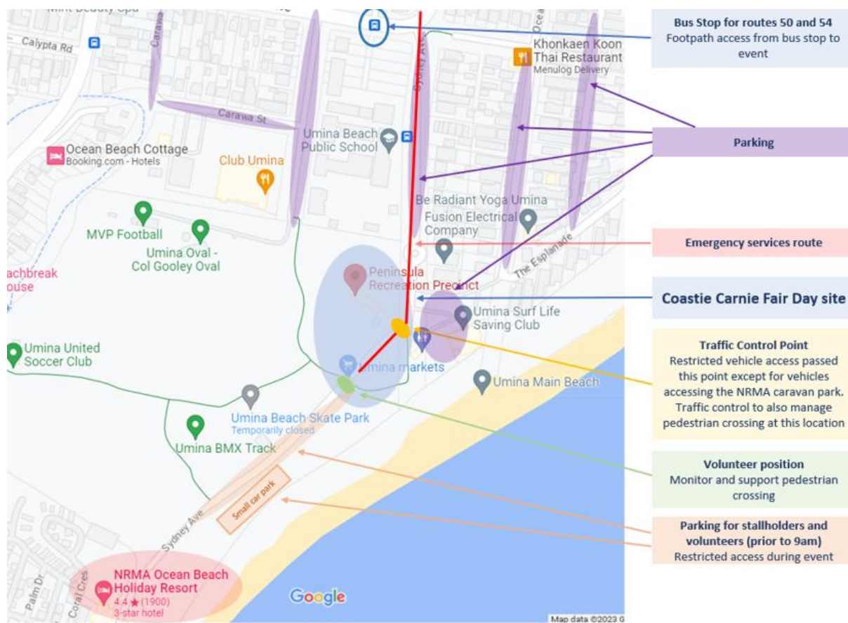
Figure 10-1: Traffic Control Layout (Preliminary TCP)
