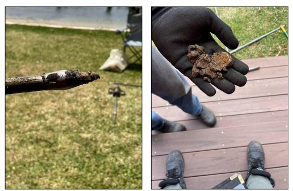
Photographs P6 and P7 – Detail of DCP probe tip on removal, and test spoil taken at test location BH1, respectively
