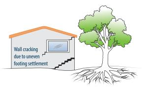
FIGURE 1 Trees can cause shrinkage and damage.
