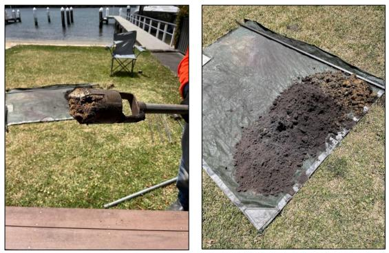
Photographs P8 and P9 – Detail of spoil in Jarrett auger and spoil layers from test location BH1, respectively
