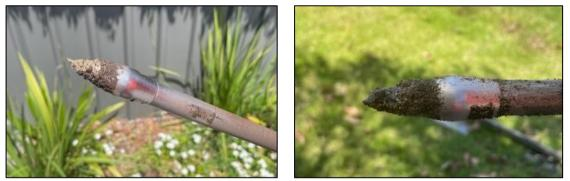
Photographs P12 and P13 – Detail of probe tip on removal, taken at test locations BH3 and BH2, respectively
